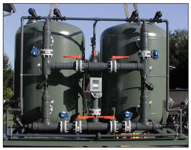
The ASDC-7272-6/2/PVC is one of our largest water softeners. The ASDC-7272-6/2/PVC features 2" regeneration and 6" outlet Schedule 80 PVC face piping, a twin alternating stager and controller which can be controlled with air or water pressure, a flow sensor, and optional flow transmitter capability. This softener also features Carbon Steel Epoxy lined ASME code tanks, Actuated PVC Butterfly valves, and Viton/EPPM seal construction.
